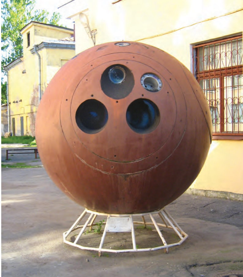
1.2 A reentry vehicle from the Zenit satellite revealing the camera ports. Photograph: Maryanna Nesina.
